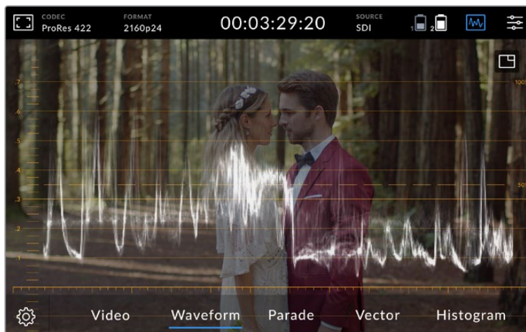
The waveform display showing luminance values
