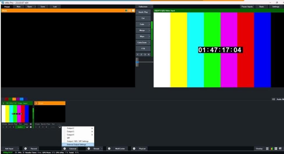
Step 2: Select "V51" as the video output device in the external output settings.
